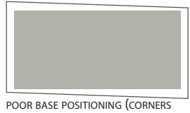
POOR BASE POSITIONING (CORNERS NOT AT RIGHT ANGLES)
